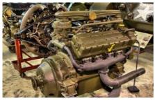
Corps a 27-litre all aluminum 60-degree V12, with four cams and forty-eight valves. The engine had some truly modern features for the time. Henry Ford was so confident he would win a major contract he already had the tooling and casting cores ordered for its manufacture.
